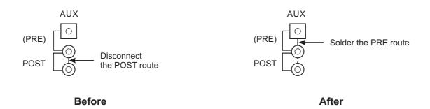
Modification on mono and stereo channels
